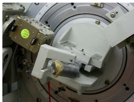
Figure 4. Non destructive XRD analyses: Bragg-Brentano diffractometer with a Goebel mirror.
