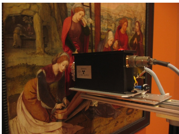
Figure 2. Analysis in situ of the panel painting by portable X-Ray Fluorescence.
